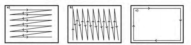
NOTE 1—Only the center of the wiping path is shown, not the entire wiping width. Fig. 2a) shows the first "Z" wiping pattern over the surface area to be sampled; Fig. 2b) demonstrates the second "Z" wiping course over the surface; and Fig. 2c) shows the final wiping which is targeted toward edges and corners.
