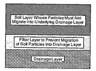
Figure 5.2 - Filter Layer Used to Protect Drainage Layer from Plugging
