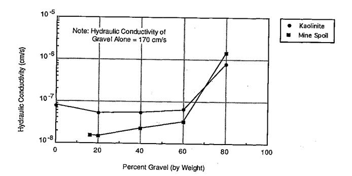
Figure 2.10 - Relationship between Hydraulic Conductivity and Percentage Gravel Added to Two Clayey Soils (after Shelley and Daniel, 1993).
