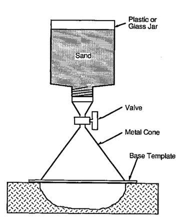
Figure 2.25 - Sand Cone Device
