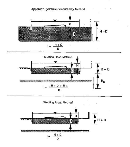
Figure 2.33 - Three Procedures for Computing Hydraulic Gradient from Infiltration Test
