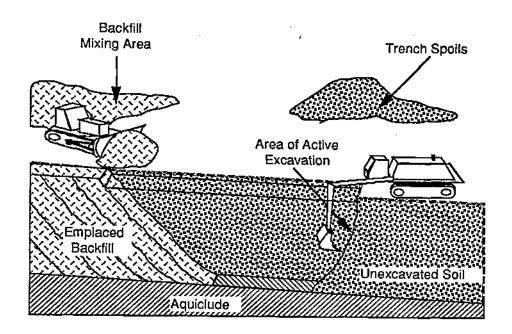
Figure 7.8 - Diagram of Construction Process for Soil-Bentonite-Backfilled Slurry Trench Cutoff Wall.
