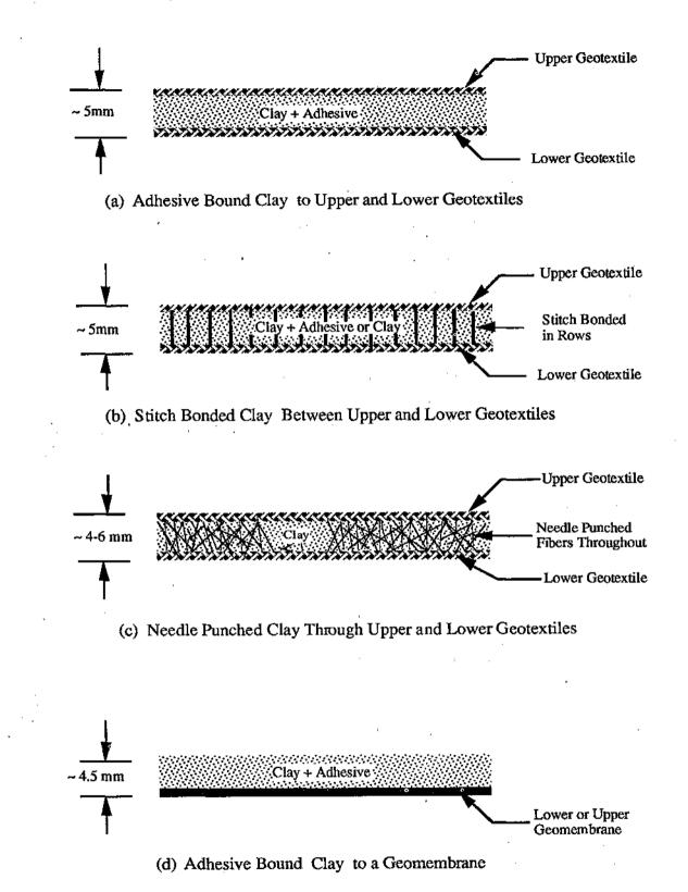
Figure 4.1 - Cross Section Sketches of Currently Available Geosynthetic Clay Liners (GCLs)
