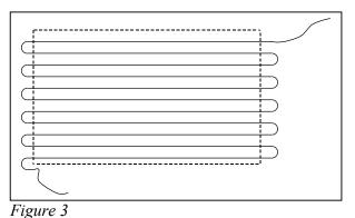
Chain folding in regular polymers. The region inside the broken line is regarded as a polymer crystal.
