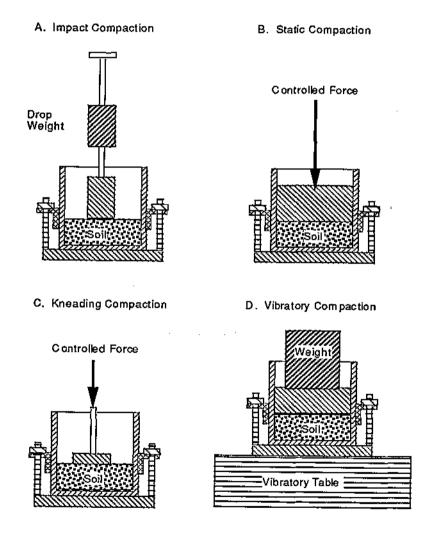
Figure 2.17 - Four Types of Laboratory Compaction Tests
