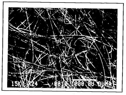
(b) Nonwoven Needlepunched Geotextile at 24X Magnification Figure 6.4 - Three Major Types of Geotextiles (Continued on Next Page).
