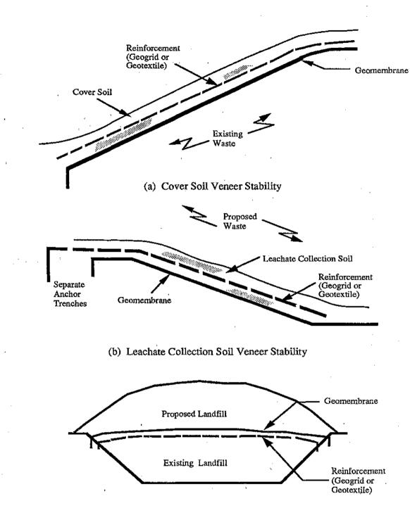
(c) Liner System Reinforcement for "Piggy backing"
