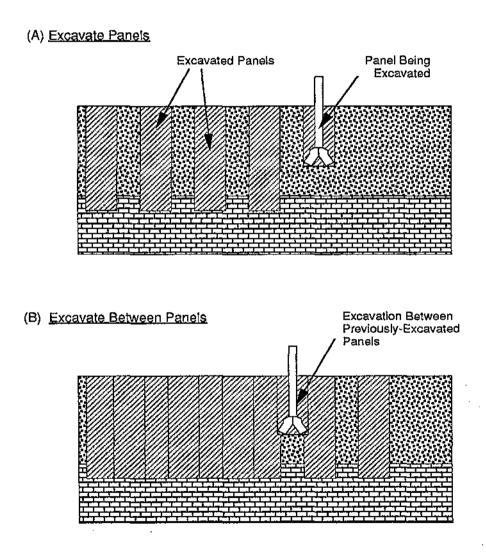
Figure 7.15 - Diaphragm-Wall Construction.
