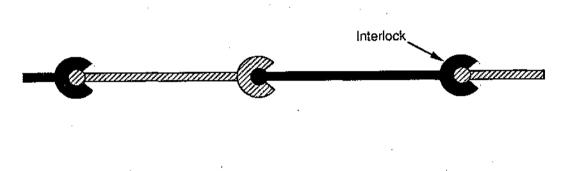
Figure 7.5 - Interlocking Steel Sheet Piles.
