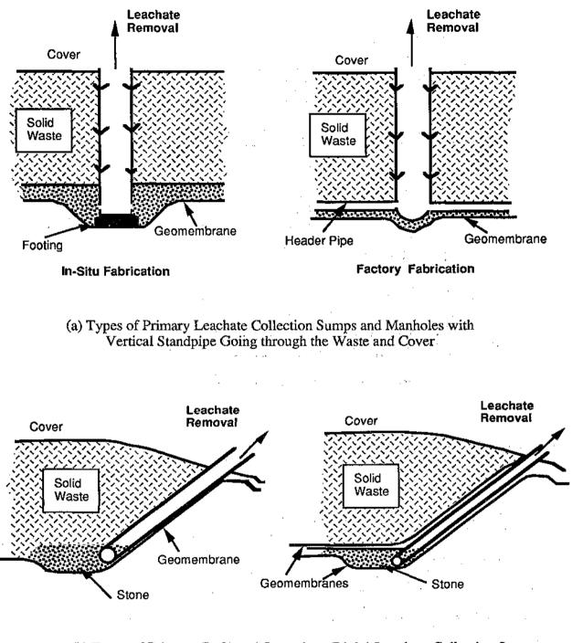
(b) Types of Primary (Left) and Secondary (Right) Leachate Collection Sumps and Pipe Risers Going Up the Side Slopes
