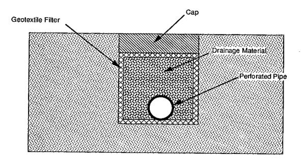
Figure 5.3 - Typical Design of a Drainage Trench
