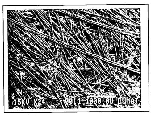
(c) Nonwoven Heatbonded Geotextile at 24X Magnification
