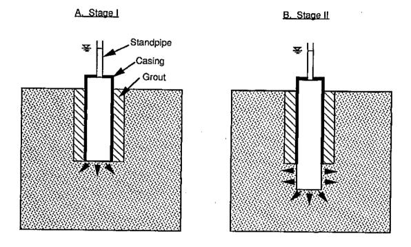
Figure 2.34 - Schematic Diagram of Two-Stage Borehole Test
