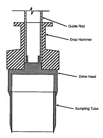
Figure 2.27 - Schematic Diagram of Drive Ring
