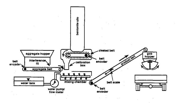
Figure 2.30 - Schematic Diagram of Pugmill
