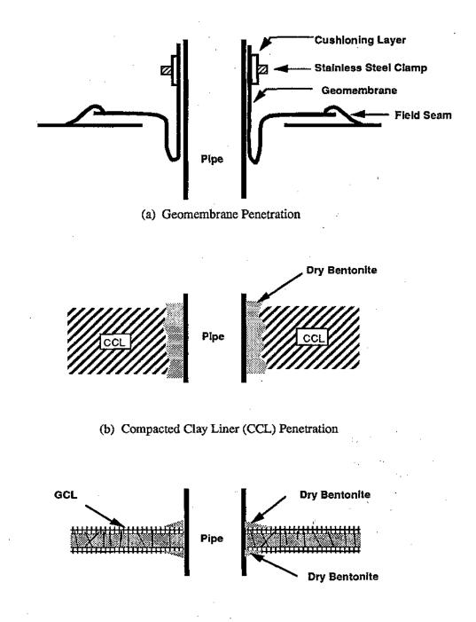
(c) Geosynthetic Clay Liner (GCL) Penetration
