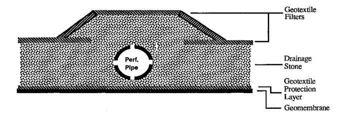
Figure 8.1 - Cross Section of a Possible Removal Pipe Scheme in a Primary Leachate Collection and Removal System (for illustration purposes only).
