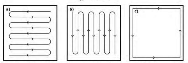
NOTE 1—Only the center of the wiping path is shown, not the entire wiping width. Fig. 1a) shows the first "S" wiping pattern over the surface area to be sampled; Fig. 1b) demonstrates the second "S" wiping course over the surface; and Fig. 1c) shows the final wiping which is targeted toward edges and corners.
