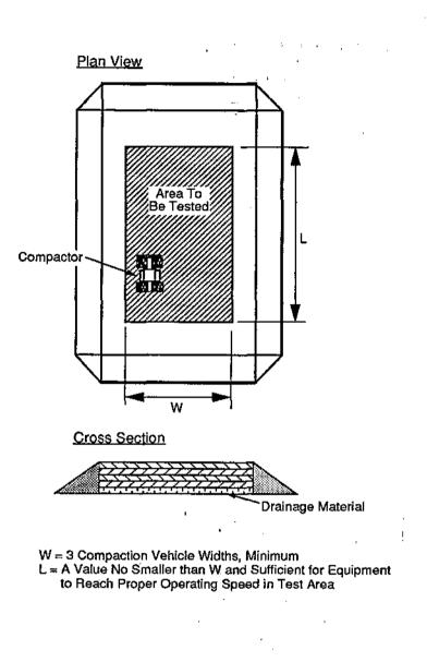
Figure 2.31 - Schematic Diagram of Soil Liner Test Pad
