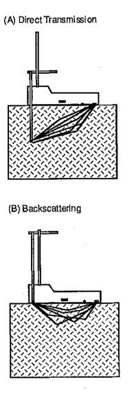
Figure 2.28 - Measurement of Density with Nuclear Device by (a) Direct Transmission and (B) Backscattering
