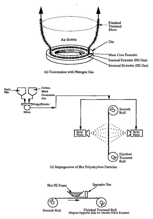
(c) Lamination with Polyethylene Foam
