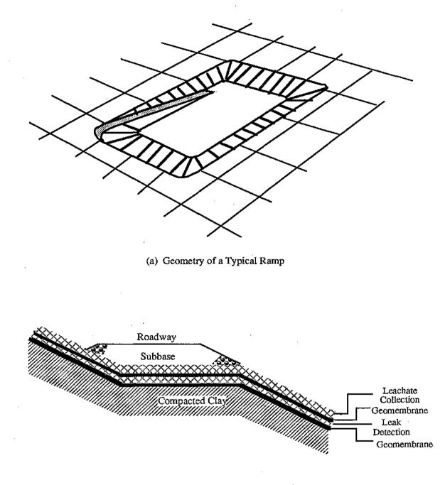
(b) Cross Section of Ramp Roadway
