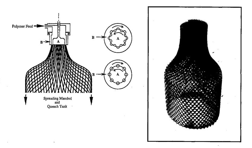
Figure 6.9 - Counter Rotating Die Technique (Left Sketch) for Manufacturing Drainage Geonets and Example of Laboratory Prototype (Right Photograph)
