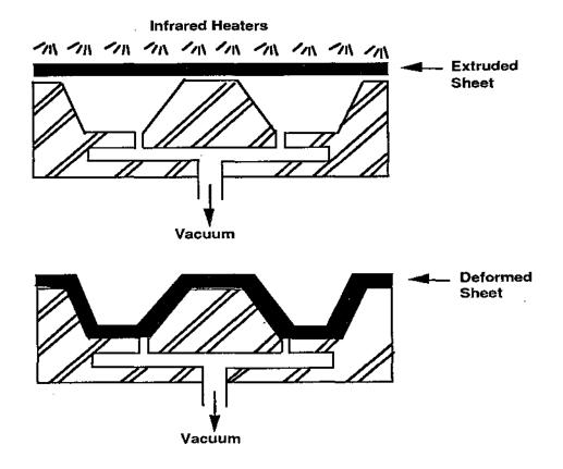
Figure 6.13 - Vacuum Forming System for Fabrication of a Drainage Geocomposite
