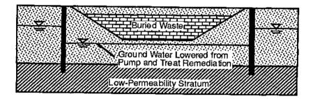
Figure 7.3 - Example of Vertical Cutoff Wall to Restrict Inward Migration of Ground Water.
