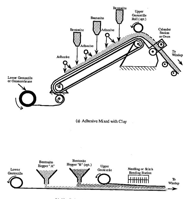
(b) Needle Punched or Stitch Bonded Through Clay
