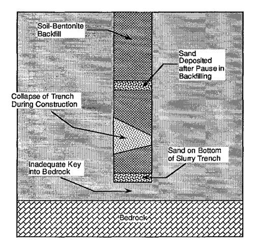
Figure 7.14 - Examples of Problems Produced by Improper Backfilling of Slurry Trench.
