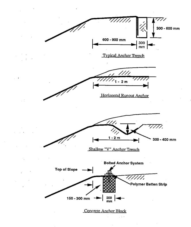
Figure 8.9 - Various Types of Geomembrane Anchors Trenches (Dimensions are Typical and for Example Only).
